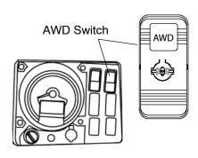
When the *RANGER* 6X6 AWD switch is in the off position, the vehicle is in two-wheel drive at all times.
